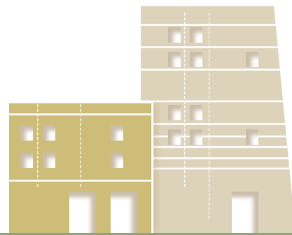
FIG. 32 General asymmetrical facades with localized symmetry in opening placement
