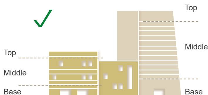
FIG. 36 Facades divided in three parts - top, middle and base. Grounded solid base with inclined walls towards the top
