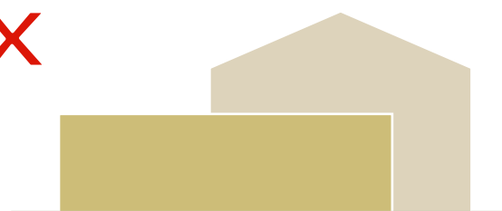
FIG. 30 Large monolithic building blocks, non contextual roof profiles should be avoided
