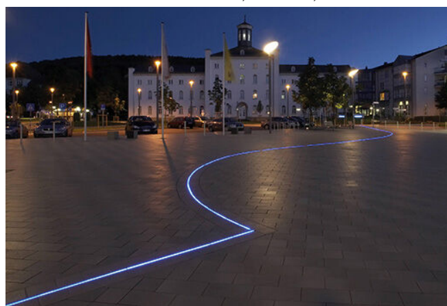
FIG. 75 Led lighting integrated in paving as a special design / wayfinding feature. Iserlohn, Germany
